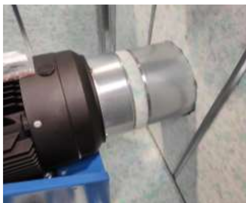
Cooling air direct drive
